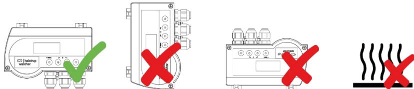
Installation in the immediate vicinity of heat and radiation sources (e.g. radiators, solar radiation...) should be avoided, as this can lead to measurement errors.
