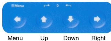
In the navigation of the device, a distinction is made between menu level and display mode. The function of the buttons varies depending on the active mode.
