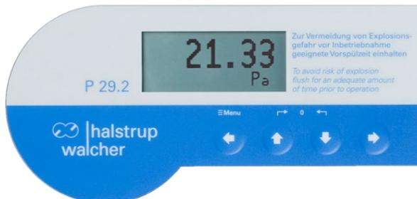
In *Display* the current measured value (or min. value or max. value) is displayed. The displayed value can be parameterized individually. See chapter **5.7 Display settings (optional)**
