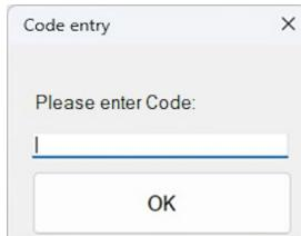
If Access Protection (see **6.8 Device settings**) is enabled, a code (numeric, 0-999999) must be entered before accessing certain features.
