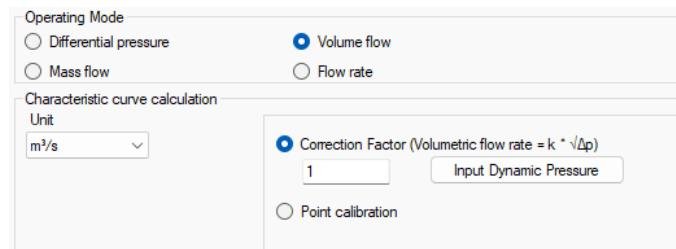
The **correction factor** can be determined in advance with the help of the manufacturer's specifications / design of the system and then entered manually in the software.
