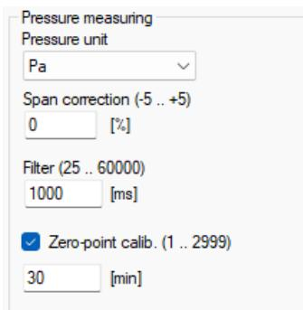
In this field, basic settings for differential pressure measurements and the zeroing interval can be made. The following options are available:
