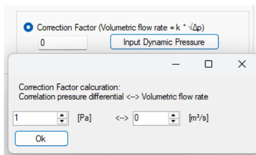
Alternatively, the **correction factor** can be calculated directly in the software. For this purpose, the ratio between a measured differential pressure and the corresponding reference value (volume flow, mass flow rate or flow rate) is used:
